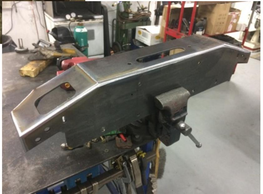
If you also purchased D-Ring tabs at this time, you can bolt them up to your welded bumper, and weld the 2 pieces per side together now. See photo for orientation. Slide the 3/4" tab and bottom plate together so the edges just touch, and weld together (be sure not to weld through to the bumper itself, unless you are permanently adding them on).
