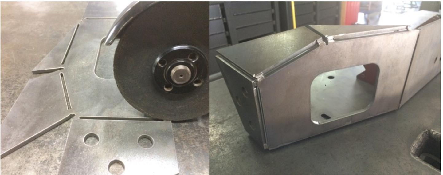
Step 3: Bend all sections of the bumper to the final shape (Note: If a piece cracks off don't worry, just realign and tack weld in place), As you are bending the bumper, pay special attention to the outermost vertical flange with 3 bolt holes. You want this to be as close to parallel with the matching cut on the bottom plate, as this is the face your frame mounts, D ring (and bumper wings) bolt to, so it being square is important.
