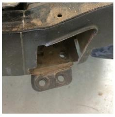
**Step 8:** Preparing to install the 6 bolt under-frame reinforcement, you will be required to unbolt the frame side sway bar mounts. It is recommended to do one side at a time so full removal is not necessary. We do recommend keeping these bolts loose to allow adjustment as the bumper and inner mounts are located, to be tightened later. 2 M10 bolts are supplied for the factory skid plate holes.
