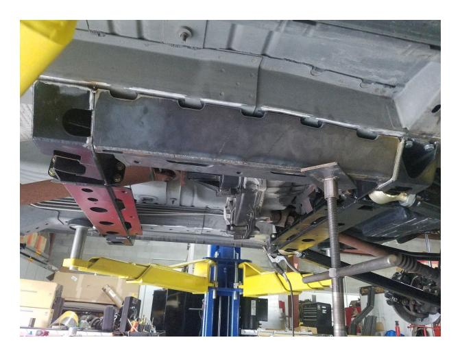
Once the welding is done, the biggest part of the installation is complete. The crossmembers and rail reinforcements can now be prepped and painted while other work goes on. This is a good time to complete the modification of your exhaust system.
