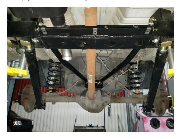
Once the front and rear suspension are installed, every recently installed nut and bolt have been torqued and everything looks satisfactory, you can install the nut clips on the subframe's skid plate mounting tabs, lift the skid into position and install with the coarse thread 3/8"-16 1.5" long flange bolts. These bolts have some extra length to make sure it's easy to grab the threads of the clip nut and pull the skid up into place with no hassle.
